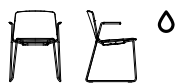
Slide frame with armrests - stackable L 55 P 54 H 78 cm W 21 5 / 8 " D 21 2 / 8 " H 30 5 / 8 "
