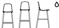
Stool with high back - aluminium base L 49 P 58 H 101-111 cm W 19 2/8 " D 22 7/8 " H 39 5/8 -43 5/8 "
